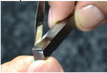
A planing scrape is shown using any one of the four 90° edges.
